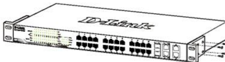
Figure 2 – Attach the mounting brackets to the Switch
